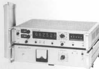
Hewlett-Packard scaler, high-voltage power supply and scintillation detector
